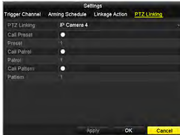
Figure 8-7 Set PTZ Linking of Alarm Input
