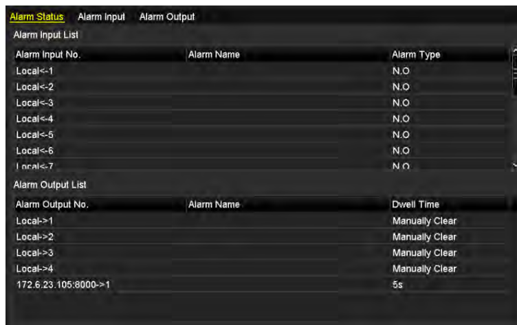
Figure 8-4 Alarm Status Interface of System Configuration
